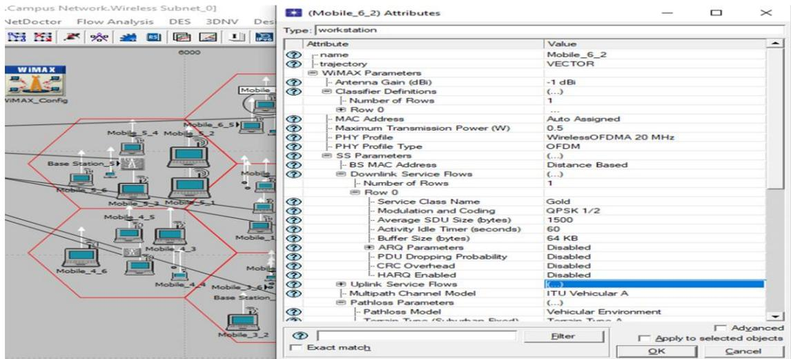
Figure 4: WiMAX Parameters Configuration and Simulation Page
