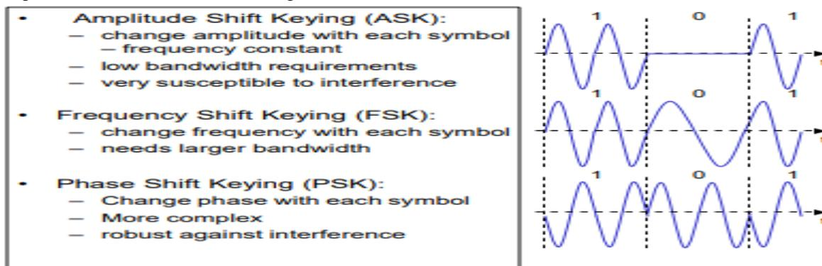
Figure 2: Digital Modulation Techniques
